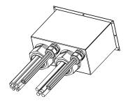
2. Connect the communication cable to the corresponding port. GRID,GEN and Back-up Fix the cables according to conductor marks of L1,L2,L3,N and PE.
