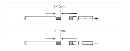
4. Assembly the positive and negative cables with corresponding crimping pliers.
