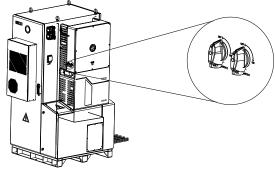
8. Connect the positive and negative connectors into positive and negative DC input terminals of the inverter, a "click" should be heard or felt when the contact cable assembly is seated correctly.
