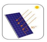
In order to achieve maximum annual yield, optimum orientation and tilt of PV modules is necessary. Sunlight shining vertically onto the PV module is the best condition to generate maximum power.
