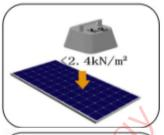
The maximum load on module must not exceed 2.4KN/m<sup>2</sup> Site-specific environment loads such as wind and snow should be taken into account to avoid exceeding the maximum.
