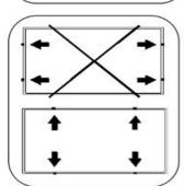
Each module should be fixed at least 8 points on long frame or short frame.
