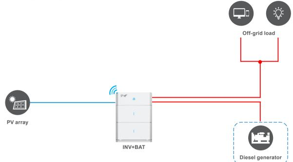
In some areas without power grid, such as ocean islands or remote areas, Kehua Energy Storage System can be combined with generators to form a complete off-grid system to ensure energy independence.
