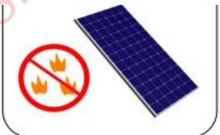
The module must not be installed close to fire or Flammable materials.
